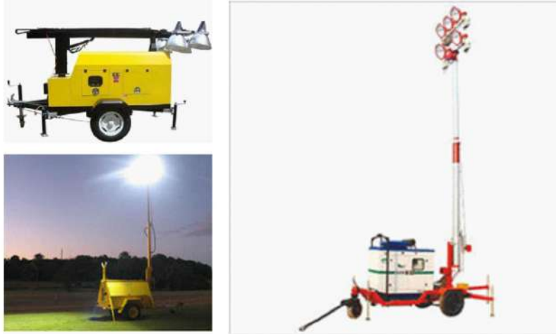
Figure 3 : Flood relief measure - To station mobile tower light facility.
